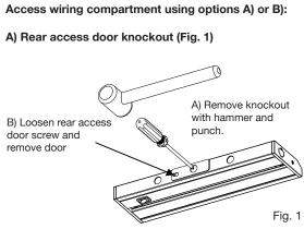
When utilizing alternative knockouts, the wiring compartment cover must be removed. Remove two screws on each end with a Phillips head screwdriver and pop off cover.
